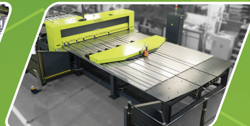
Fully automated cutting centre with CNC pre-stop and conveyor system
