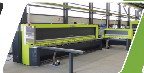
Right-angled setup for easy cutting of long sheet metal
